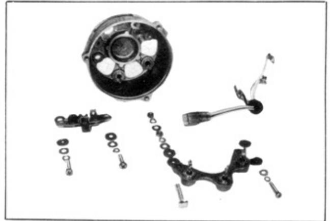
Remove the diode set and brush holder from the rear cover.
