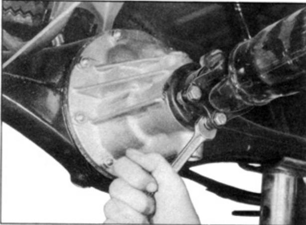
Before disassembling, mark all components of shaft so as to assemble them in the former position and avoid that the propeller shaft balance may be some how affected.
