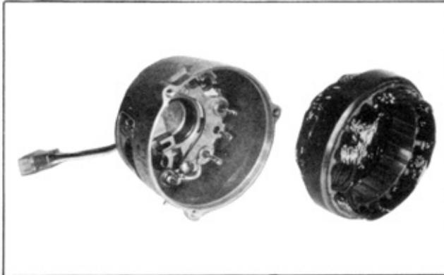
Remove the rear cover and stator.
