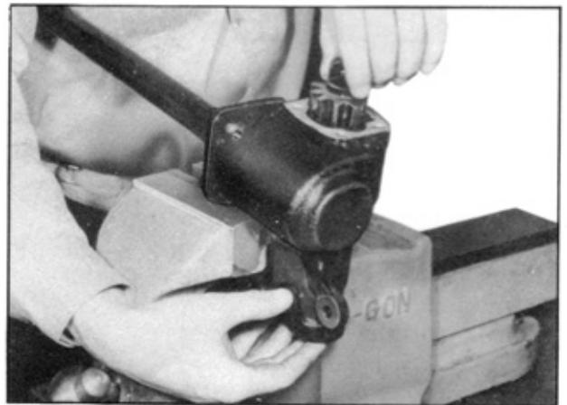
Separate the adjusting screw and the side cover and detach the sector shaft from body.
